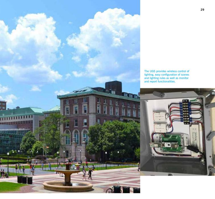
functions. The combination of the UGS with self-powered lighting controls based on energy harvesting technology enables the definition of lighting scenes and rules which allows enormous energy and cost savings. For example, presence sensors can be used to determine whether a room is occupied or not. If no student is present, the system turns off the lighting and enables energy-efficient operation.
