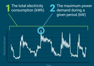
To reduce cost related to maximum demand, common load shedding technologies prevents the most energy-consuming equipment to operate simultaneously.
